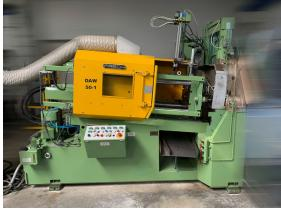
A large industrial machine, specifically a Frech DAW 50 pressure casting machine. It features a prominent yellow hot chamber unit mounted on a green base frame. The machine is equipped with various mechanical components, including a flywheel, belts, and a control panel with multiple buttons and a small display screen. | <b>1,00 €</b>   |
